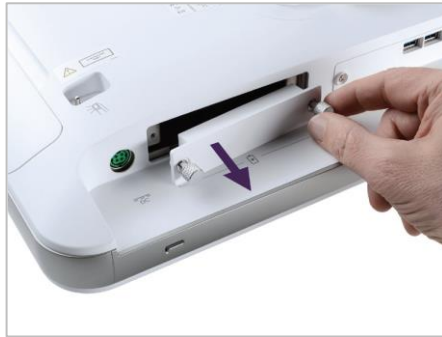
10. Loosen the thumbscrews and remove the battery cover.
