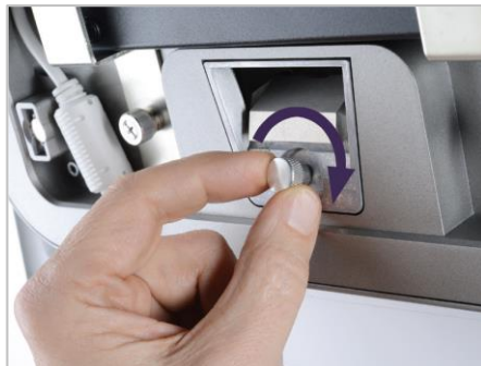
13. Turn the scanner around and tighten the thumbscrew to secure the screen.
