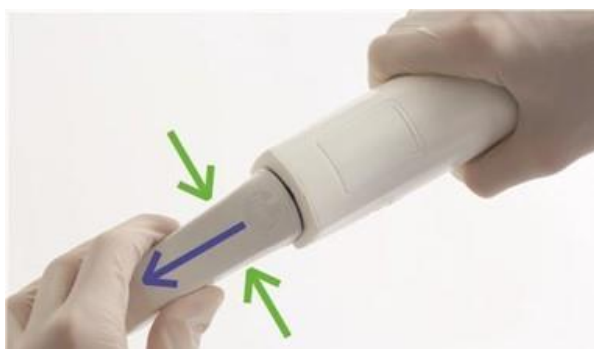
Figure 8: Removing a wand sleeve
