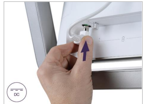
14. Connect the power cable to the port labeled DC, as shown in the next image.
