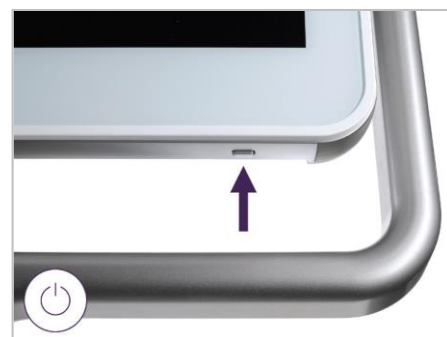
22. Plug the power cable into the AC power outlet and then press the Power button to switch on the scanner.
