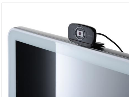
20. Position the webcam on the touch screen for remote training or support sessions.
