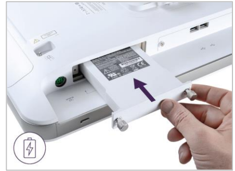
11. Slide the battery into the battery slot and tighten the thumbscrews.
